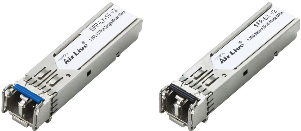
The SFP-LX-10 v2 is a high performance and cost-effective module for serial optical data communication applications specified for singlemode of 1.25 Gb/s. The module is intended for single mode fiber, operates at a nominal wavelength of 1310nm. The module is a duplex LC connector transceiver designed for use in Gigabit Ethernet applications and to provide IEEE802.3z compliant link from 125Mbps to 2.125Gbps applications.
